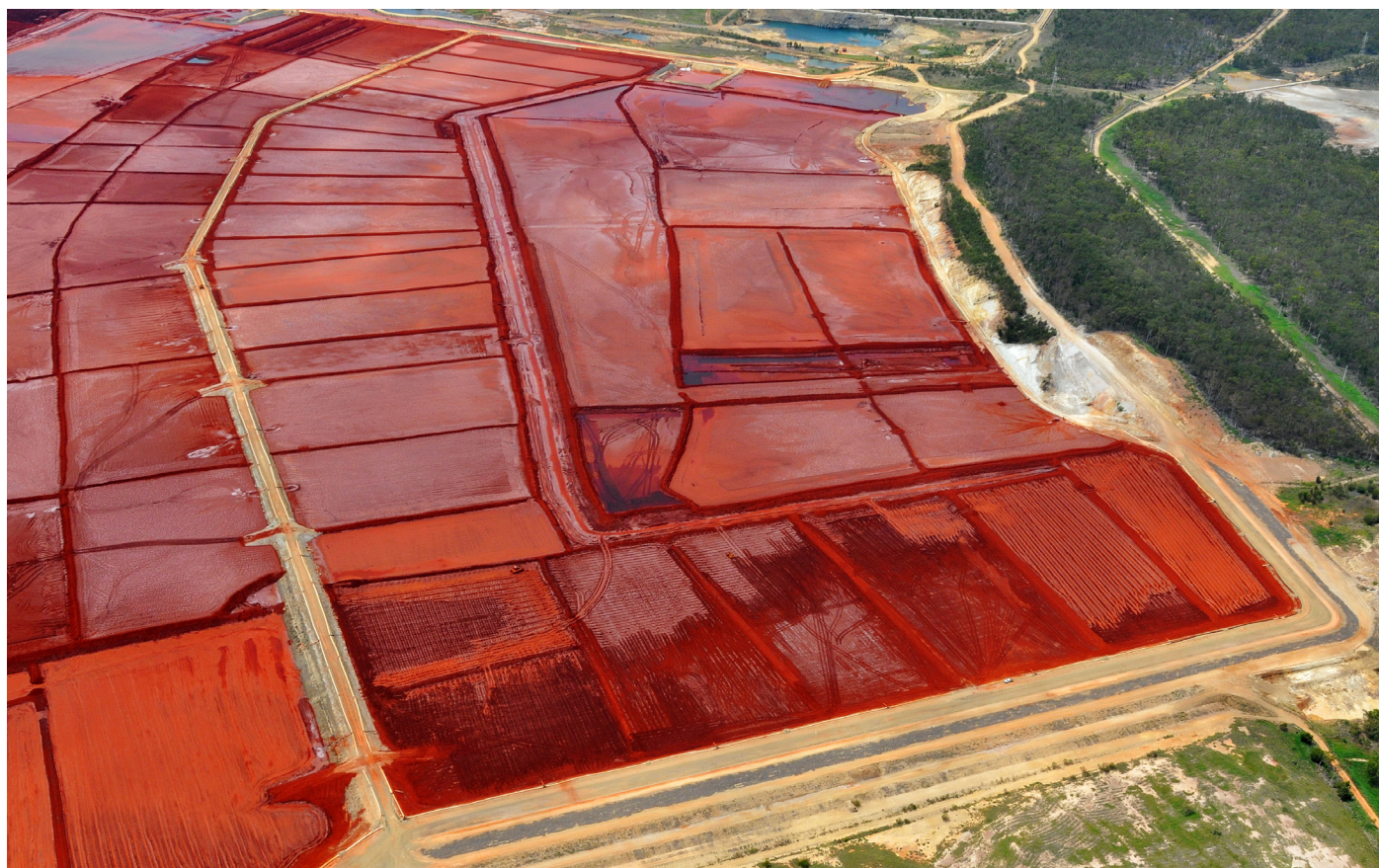
Figure 14. BRSF divided into bays, where it is deposited, farmed and dried sequentially.
