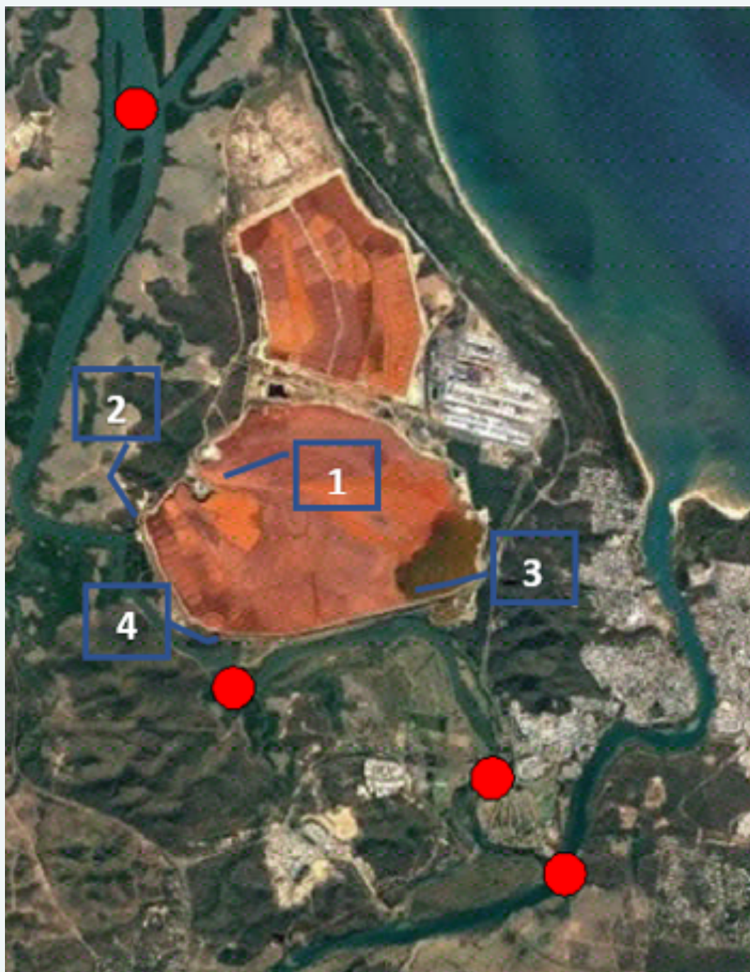
Figure 3 1. Neutralisation Facility 2. Seawater Intake 3. Labyrinth and diffuser 4. Discharge point ● Continuous Monitoring Points
